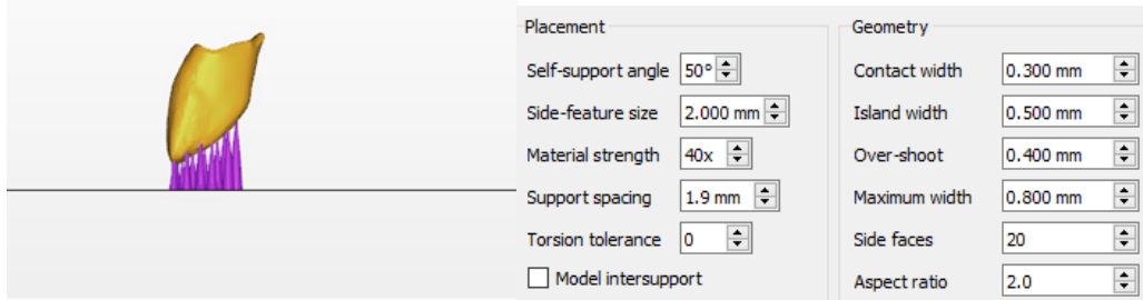
Fig. 3-4: Positioning of telescopes (yellow) with supports (pink) and recommendation for setting the support parameters
